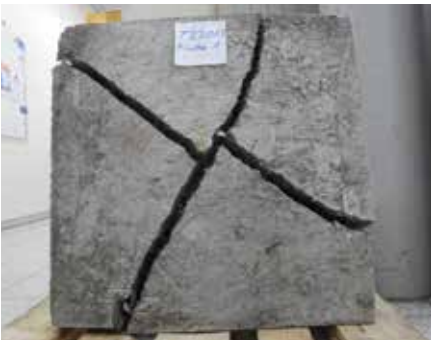
Figure 8.2.1.2: Underside view of tested square panels
