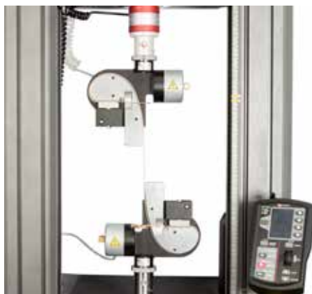
Figure 4.4.1.2: Snubbing clamp referred to ASTM D 2256-02
